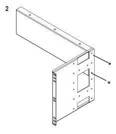
Use (2) M4 screws to mount ear bracket to first panel
