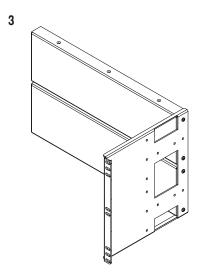
Place 2nd panel below the top panel. Use (2) M4 screws to secure 2nd panel.
